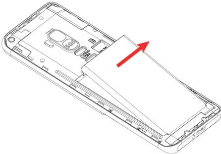
7. Replace the back cover by sliding and pushing your fingers across the edges of the back cover to ensure it has completely clicked back into place.
